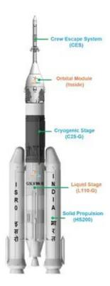
**Orbitual module** - Orbital Module (OM) that will be Orbiting Earth comprises of Crew Module (CM) and Service Module (SM). OM is equipped with state-of-the-art avionics systems with adequate redundancy considering human safety.
