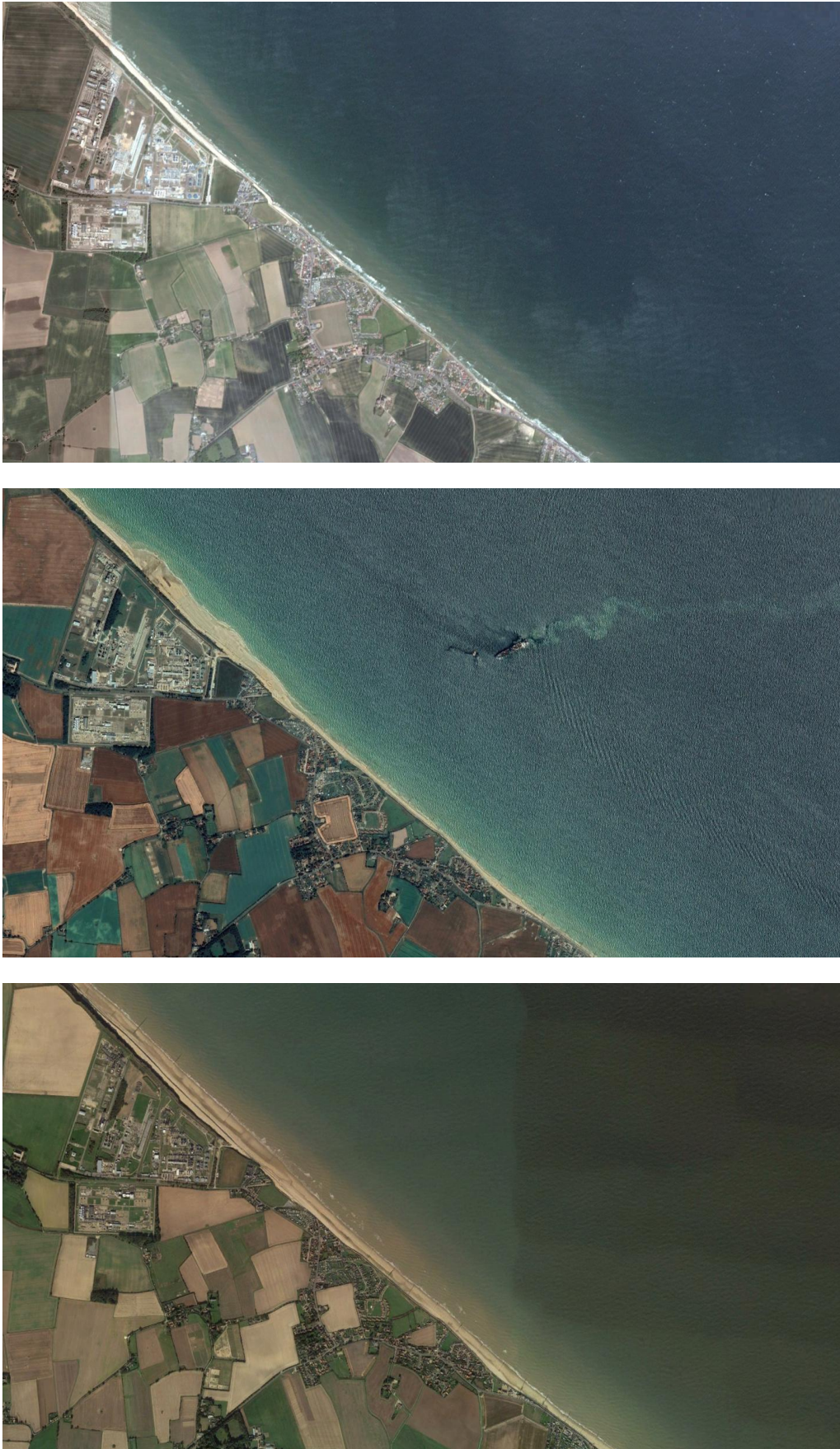
Figure 10-6: The Bacton to Walcott Coastline Prior to Sandscaping (Top, May 2011), During Sandscaping (Middle, July 2019), and After (Bottom, October 2024) [Source: Google Earth]
