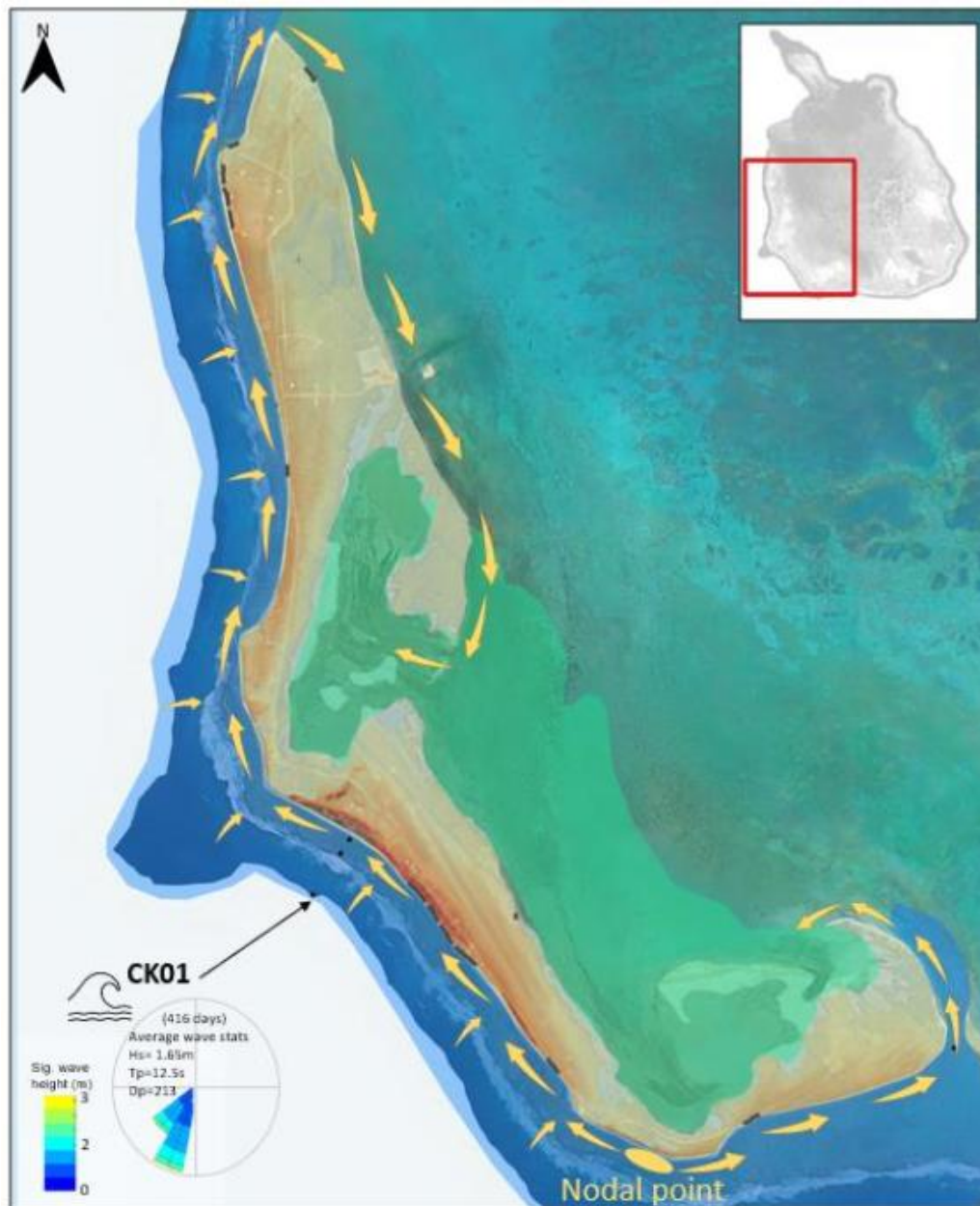
Figure 10-3: Conceptual Coastal Processes Model for the West Island (CVA Figure 64)
