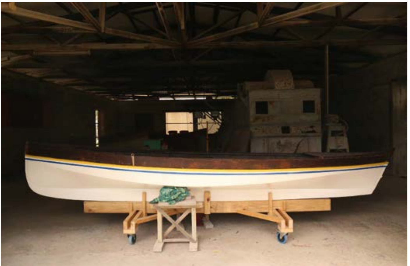
Lantar Pujeh on support frame - Chocks in place while Nek Ainul installs the hull supports.
