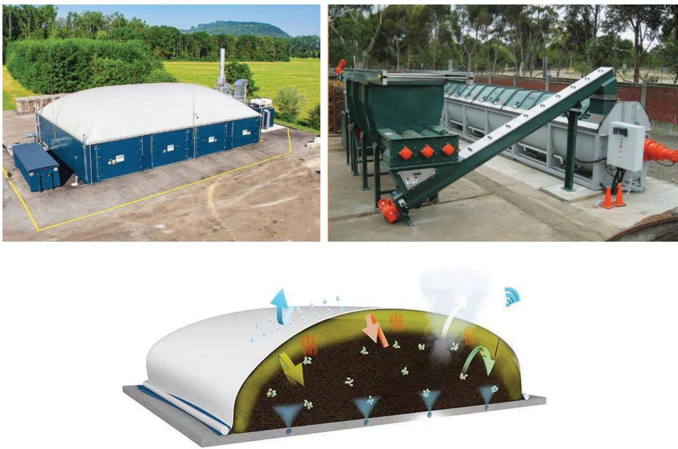
Figure 6.8 High solids 'dry' anaerobic digestion facility (Bekon, 2018) (top left), HotRot in-vessel composting system (Global Composting Solutions, 2022) (top right) and Biodrying concept by Eggersmann (bottom)
