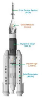
**Orbitual module** - Orbital Module (OM) that will be Orbiting Earth comprises of Crew Module (CM) and Service Module (SM). OM is equipped with state-of-the-art avionics systems with adequate redundancy considering human safety.
